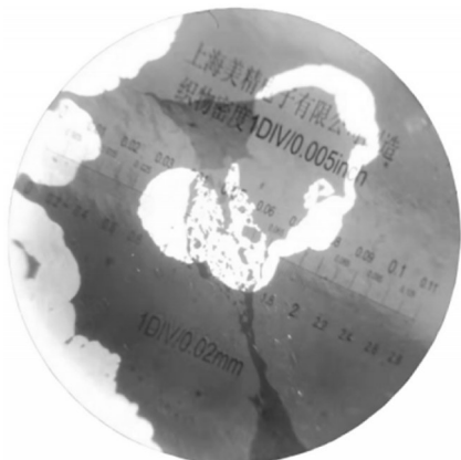
图6 金属层氧化缺失 Fig. 6 Lack of oxidation in the metal layer
